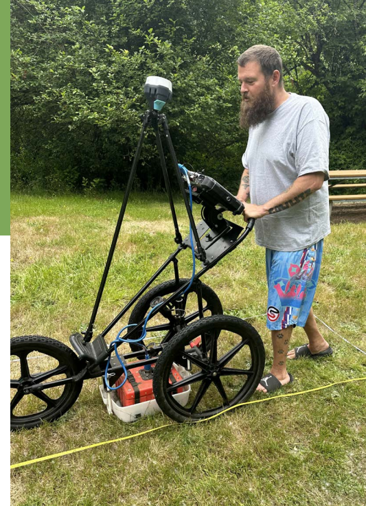
Jeremiah Wallace pushing a Ground Penetrating Radar for a project on Cowlitz homelands.
